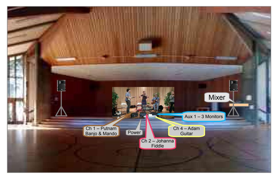
Speakers should be something like this on the stage with the tilters in place at 7°. Run them up at full mast. Use sand bag on base. Run power from outlet downstage center with right angle adapter.
